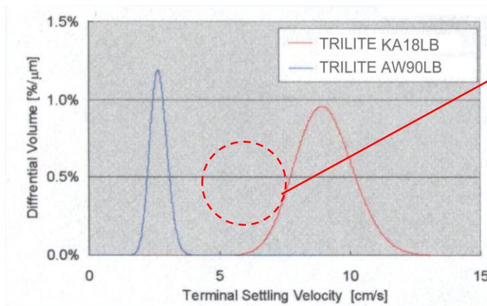
**Sedimentation rate of TRILITE KA18LB is much faster than that of AW90LB. Uniformity of TRILITE AW90LB results sharp rate of differentiation for sedimentation. Hence, there is no mixture of 2 types of IERs.**
