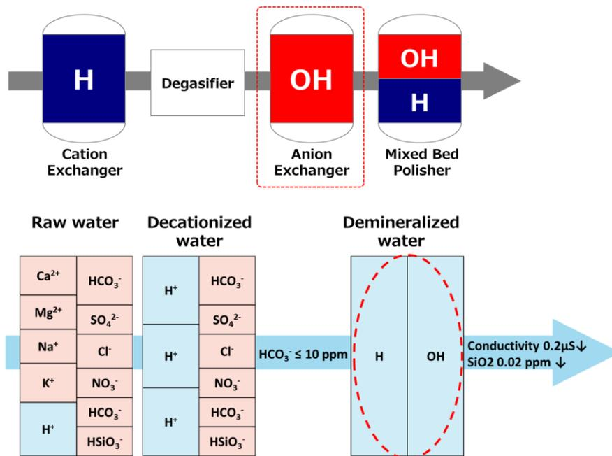
The 2B3T+MBP system, a typical demineralizer using SAC and SBA ion exchange resin, is shown in the figure above. The layered bed system employs two types of anion exchange resins in the anion exchanger.
